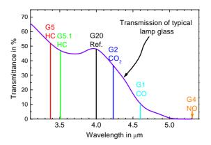
Figure 10: The curve shows the transmission characteristics of a typical lamp glass together with the center position of some gas absorption bands. The intensity of the IR light decreases above 4  $\mu$ m with a cutoff wavelength, which is located at 5  $\mu$ m. The CO<sub>2</sub> absorption is still well within a high intensity region, whereas the detection of CO is already extremely difficult due to the limited IR output.
