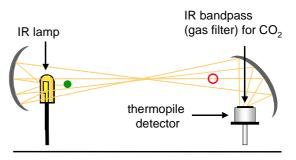
$\bigcirc$  CO<sub>2</sub> Molecule  $\bigcirc$  Other Molecules Figure 1: Schematic sketch of an infrared absorption gas detector. The to be detected gas is CO<sub>2</sub> in this example.
