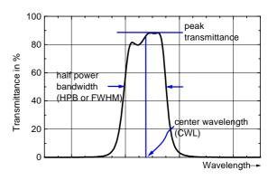
Figure 6: Visualization of characteristic IR bandpass filter parameters.
