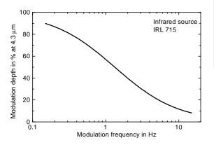
Figure 11: Modulation depth at 4.2  $\mu$ m as a function of modulation frequency of the IR source IRL 715. The resulting curve shows a typical low pass behaviour with a thermal time constant of 290 ms. (Remark: the time constant for radiation in the visible spectrum as sometimes stated in data sheets is considerably shorter.)
