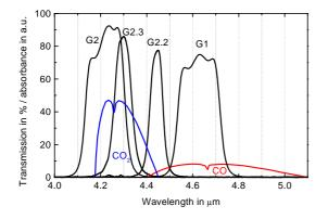
Figure 8:  $CO_2$  and CO absorption regions (schematically sketched for high concentrations) together with the position of some PerkinElmer IR filters for these gases. The relatively broad G2 filter covers most of the  $CO_2$  absorption region. G2.3 is placed on the strongest lines. The filter G2.2 is located in a region, where the absorption strength already approaches that of CO.
